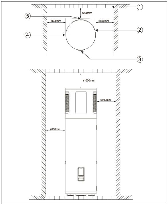
[1] Wall [2] Condensate drain outlet [3] Control panel [4] Air inlet [5] Air outlet
